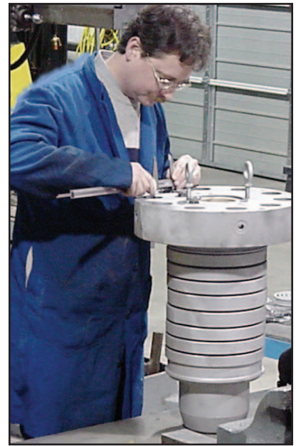
■ This gas storage packing case for an I-R KVS-512 is being double checked prior to shipment to the customer. Valves and cases are checked against minimum design standards, magnetic particle tested for cracks, and reconditioned to like-new condition. New internals are installed and the assemblies are then leak tested, CNC stenciled, packaged and labeled.
