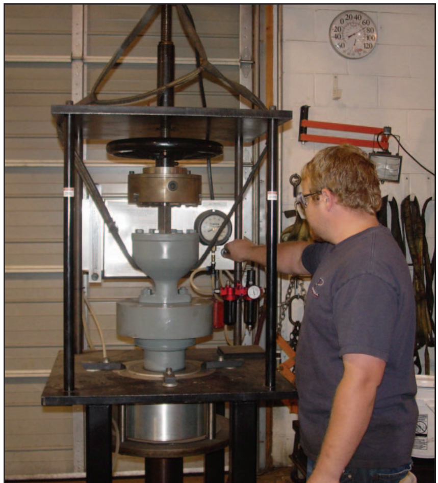
A Hi-Tech technician conducts an air leakage test on a rebuilt compressor unloader prior to returning it to a customer for installation on a Worthington BDC compressor in hydrogen service.
