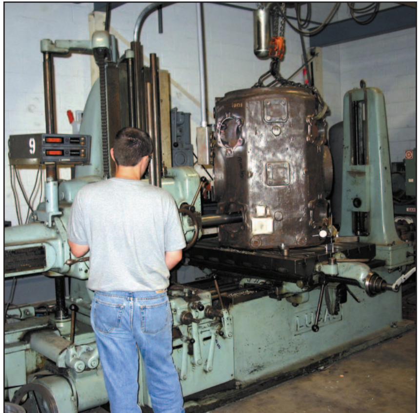
■ A local refinery discovered during a turnaround that this 13.5 in. (342.9 mm) diameter, 10.5 in. (266.7 mm) stroke Cooper Bessemer FM-2 hydrogen cylinder had cracks and pulled studs around a valve pocket. Hi-Tech metal stitched the casting, installed a sleeve in the valve pocket, restored dimensions and hydrostatically tested it to 1.5 times the maximum working pressure. They then rebuilt the cylinder with refurbished valves and new wear parts, returning it to the customer in only one week.
