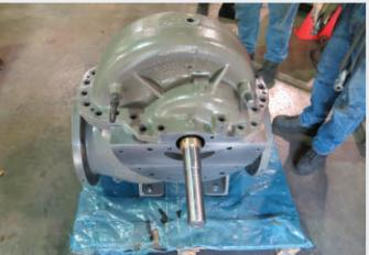
■ Hi-Tech restored the fit-up dimensions of mating parts in the assembly and applied a corrosion-resistant ceramic coating to the inside flow surface (left) as part of a complete reconditioning of this horizontally split Worthington pump (right).
