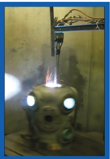
■ After ultrasonically testing the casting to confirm adequate thickness, the worn bore of this Knight KOC compressor cylinder was restored using an iron-based alloy plasma spray before it was ground back to its original size. Hi-Tech has successfully restored numerous Knight and Ariel unlined cylinders in this manner, including quick turnarounds when needed.
