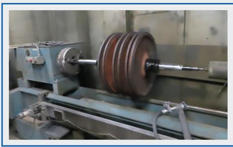
■ Hi-Tech restored the worn bearing journals on this Skinner steam turbine rotor by rebuilding them with 400 series stainless-steel thermal spray and then grinding them back to original size.
